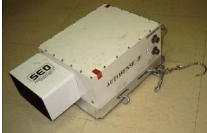
Figure 2. Autosense II Active Infrared Imaging Sensor
