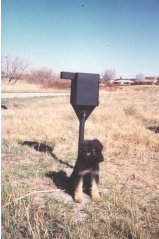
Figure 1. Infrared Laser Counter in Weatherproof Box
